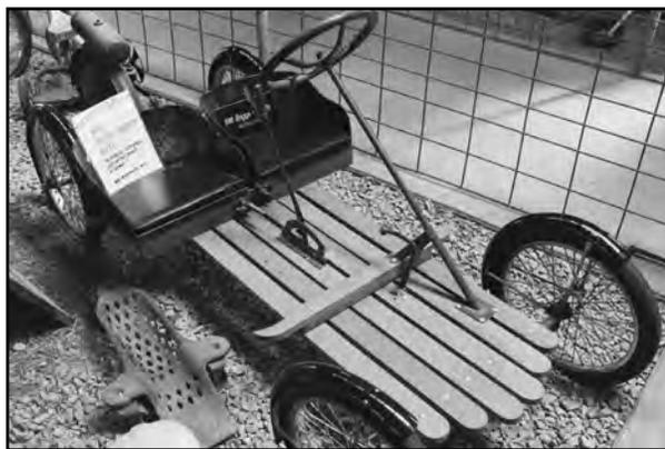
The 1918 Briggs & Stratton Flyer was hardly more than boards on wheels, powered by a small motor. It was made in Milwaukee.
